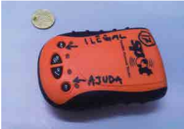
Figure 14: One button to report IUU, one for emergencies
