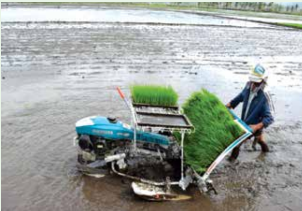
Planting of rice seedlings using mechanical rice transplanter at Mr. Abarquez's farm in Barangay Balangibang, Polangui, Albay
